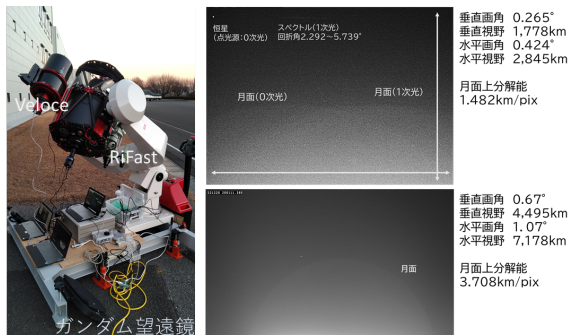
Figure 7. GUNDAM telescope, field of views and corresponding moon surface regions (12/22/2020).
